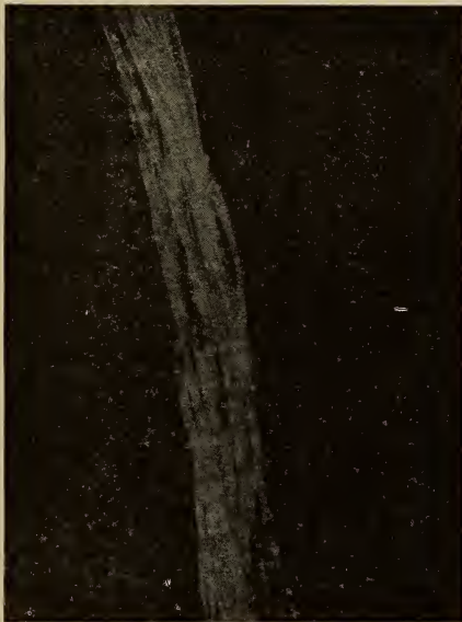
FIG. 41 SINGLE THREAD OF ARTIFICIAL SILK YARN
